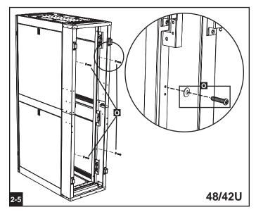
Use two M6 x 12 mm screws and washers L to connect the included grounding cable N from the rack enclosure to the extension frame.
